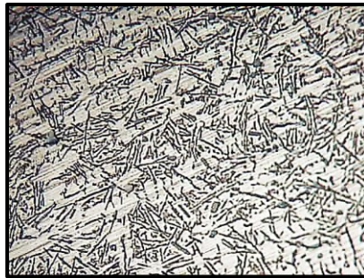
Figure. 2 shows the microscopic images of the unmodified Aluminum-11% Silicon alloys at 0 % Sb and 125 X
