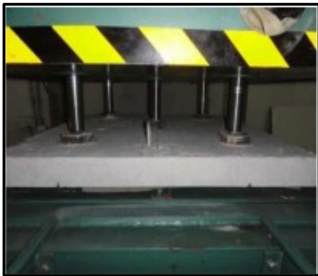
Fig. 3. Test configuration of two-way Bubble deck slab. [20]
