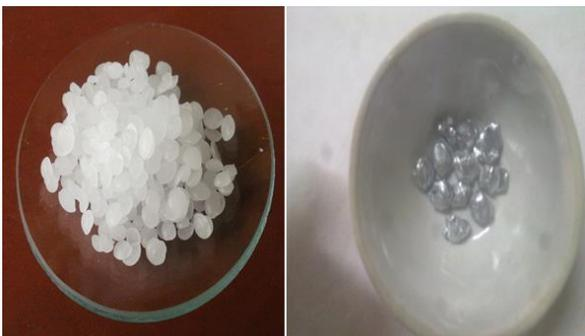
**Figure (3)** photograph of the used paraffin wax (A) Before capsulation and (B) After capsulation
