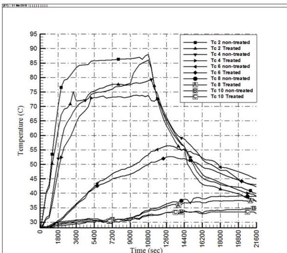
Figure (7) Comparison of temperature between the treated and non-treated walls with time
