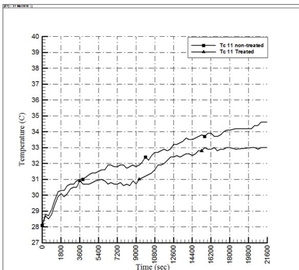
Figure (8) Comparison of internal surface temperature between the treated and non-treated walls with time
