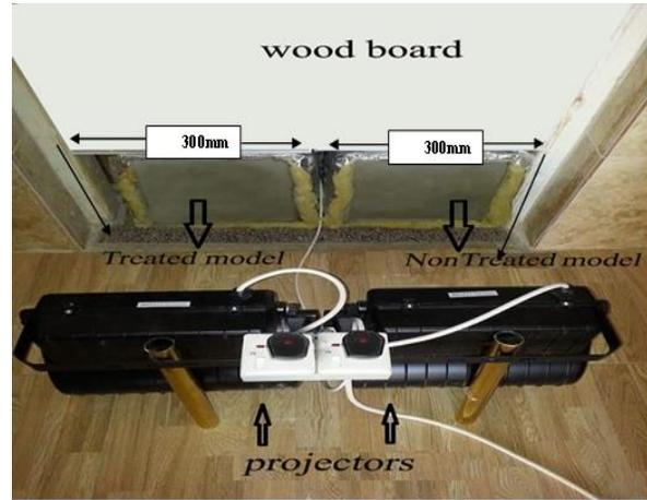
**Figure (4)** photograph of the projectors and the models
