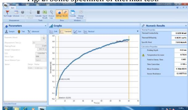
Fig. 3: The Hot Disk test results.
