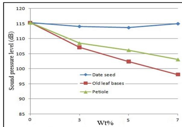
Fig. 9: Effect of filler content and type on the sound pressure level at 100 HZ frequency.
