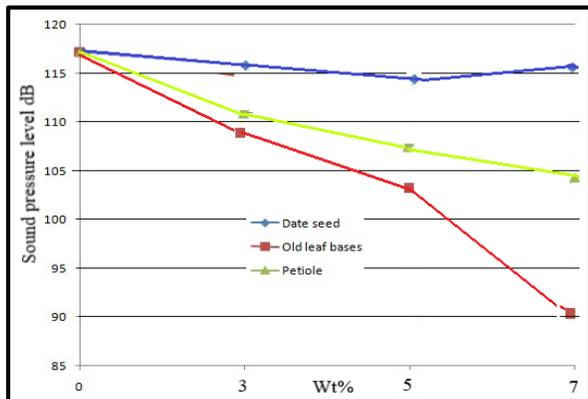
Fig. 10: Effect of filler content and type on the sound pressure level at 6 kHz frequency.
