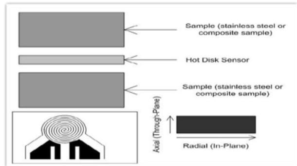
Fig. 1: The Schematic of Hot disk sensor.
