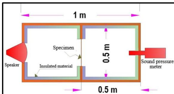
Fig. 5: The sound-insulated box.
