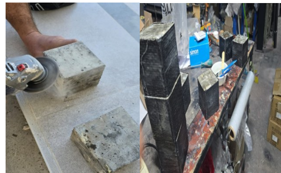
Figure 2: specimen preparation for wrapping: Figure 3: Carbon fiber wrapping procedure
