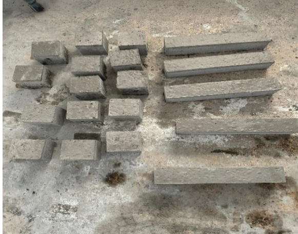
Figure 5. Prism and cube specimen
