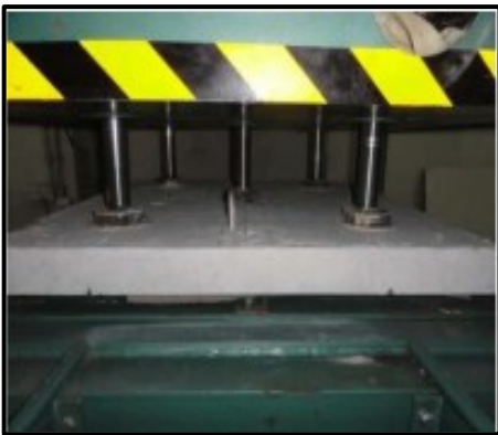
Fig. 3. Test configuration of two-way Bubble deck slab. [20]
