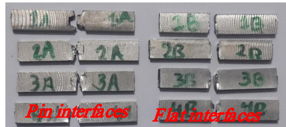
Figure 8 Specimens after completion of impact tests
