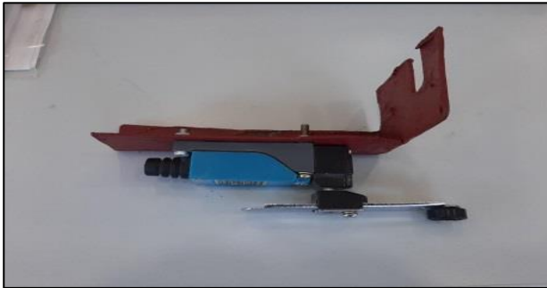
(b) A single limit switch
