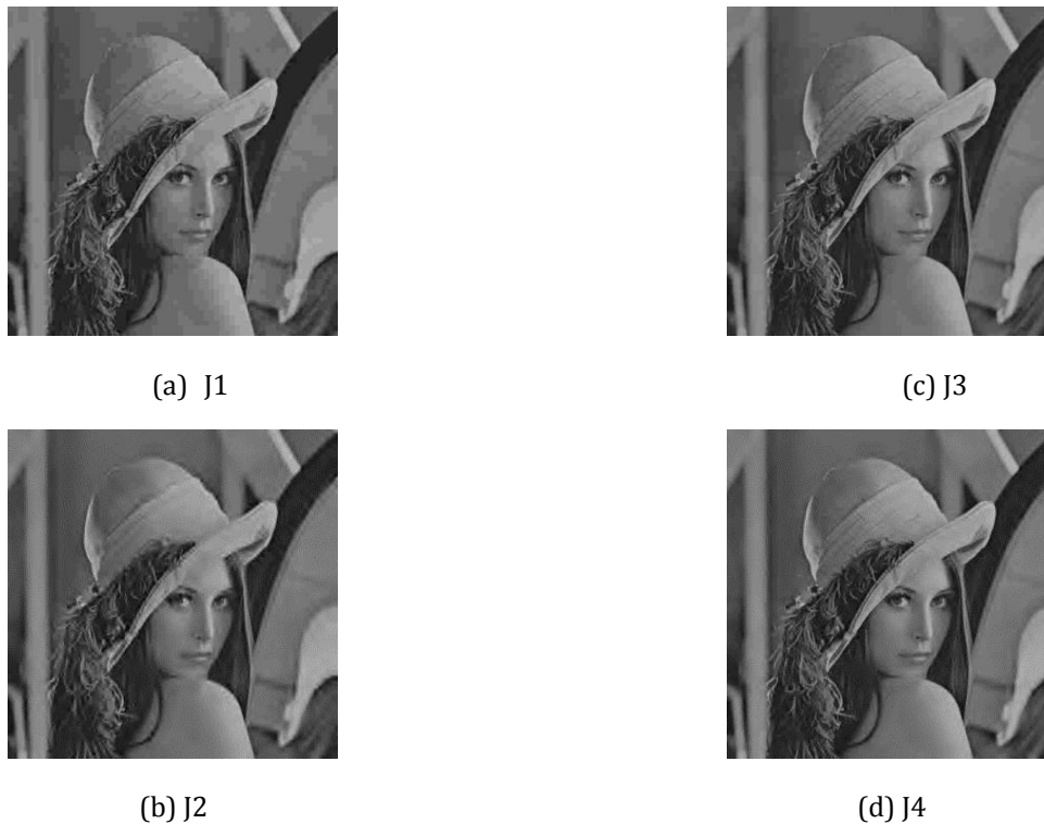
Figure 7 The subjective assessment for compressed Lena image (a) J1 is compressed using JPEG at a high CR, (b) J2 is compressed using JPEG2000 at a high CR, (c) J3 is compressed using JPEG at a mid CR, (d) J4 is compressed using JPEG2000 at a mid CR.
