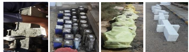
Figure 6: Casting and Curing of RCASCC Beams.
