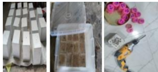
Figure 5 Chloride Penetration Test Process.
