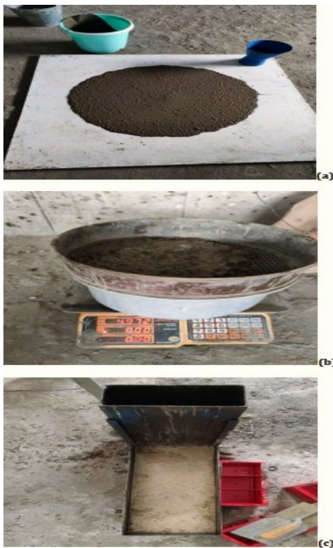
Figure 2 Fresh properties tests (a) Slump flow resistance (b) Segregation resistance (c) Blocking ratio
