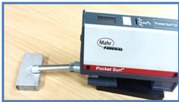
Figure 3. Pocket Surf is used to quantify surface roughness
