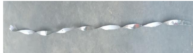
Figure 4. Perforate Twist tape insert in tube
