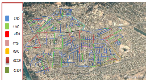
Figure 4. Storm Sewer Network in Ramadi city center as generated by Google Earth
