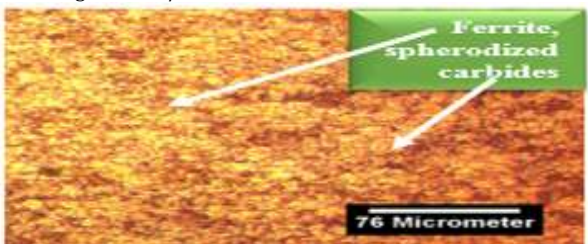
Figure 3. base- metal zone for AISI 420 MSS after annealing at 850°C/15 min.
