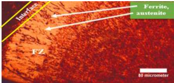
Figure 2. Fusion- metal zone for AISI 420 MSS/ ER 309L after annealing at 850°C/15 min.
