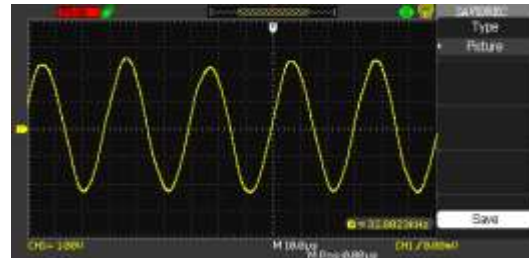
Figure 11. Output signal after receiving circuit
