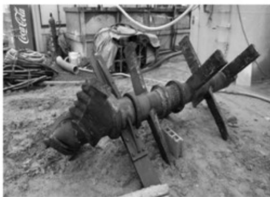
Figure 4. Mixing blades and free blade for CDM method for on-land works[6]
